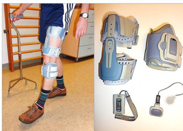
Fig. 2 The functional electrical stimulation device including two cuffs, a foot switch, and a control unit
