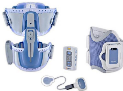
Fig. 1 The NESS L300 ® Plus neuroprosthesis system (NESS Ltd., Ra'anana, Israel), generating electrical stimulations to the quadriceps muscles
